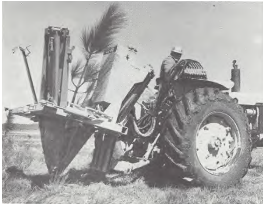
Figure 1.--A 2 year old longleaf graft being transplanted with the tree spade.
