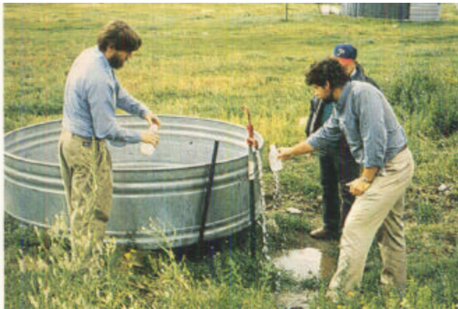
Figure 1.2.3- The first step in determining the suitability of a potential nursery site is to collect water samples from all potential sources of irrigation water and obtain a complete water analysis.
