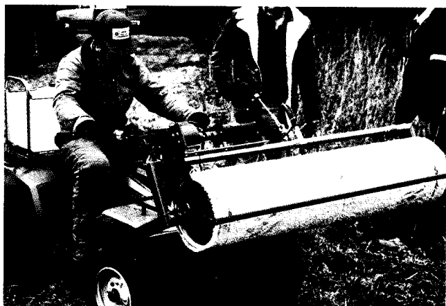
Figure 1 —Single-passenger four-wheeler mounted with a carpet-covered roller-wiper assembly. An electric motor turns the drum during application, and the chemical is added from a drip pipe mounted above the roller. The tank is mounted on the rear of the four-wheeler.
