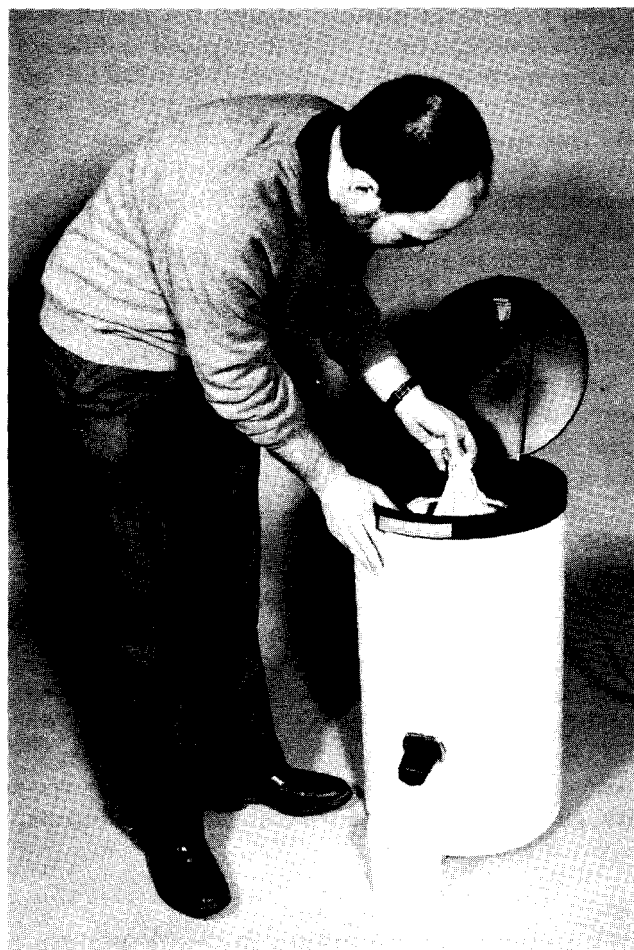
Figure 1 —Using the spin-drier to prepare soaked tree seeds.
