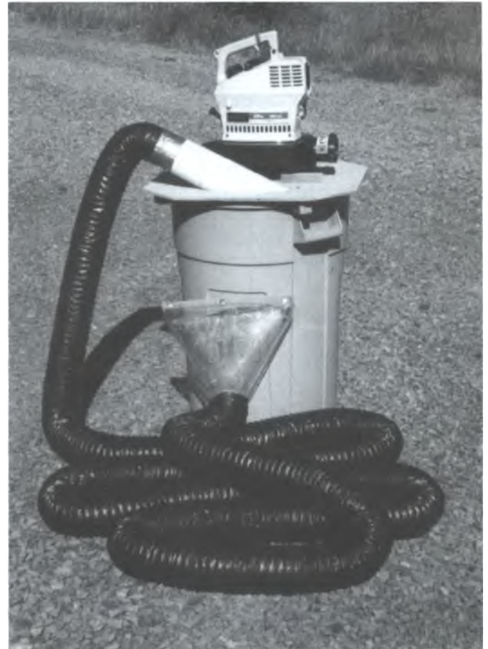
Figure 1 —Inexpensive pollen collector for small orchard needs.
