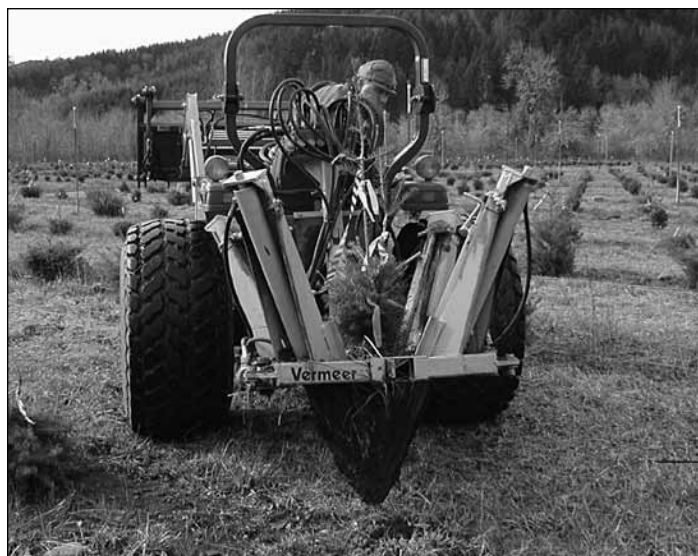
Figure 8. Moving a ramet from a holding orchard to permanent location with a treespade.
