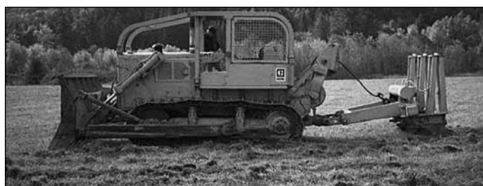
Figure 3. Using a winged subsoiler to break a hardpan in a previously cultivated property.
